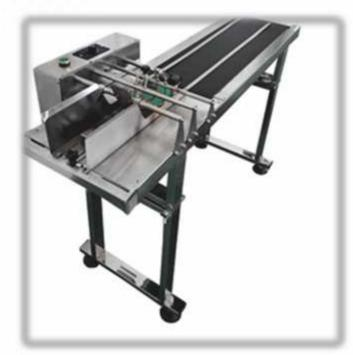
Friction feeders are ideally suited for the feeding separation and counting of flat products e.g. envelopes, phone cards, carton cuttings, inserts.
